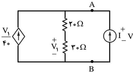
$$V = (20 + 30) \left( I + \frac{V_1}{40} \right) = 50I + \frac{5}{4} V_1$$
