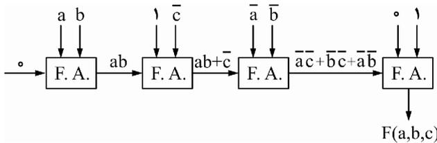
$$\Rightarrow f(a, b, c) = 0 \oplus 1 \oplus (\bar{a}\bar{c} + \bar{b}\bar{c} + \bar{a}\bar{b}) = \overline{(\bar{a}\bar{c} + \bar{b}\bar{c} + \bar{a}\bar{b})}$$
