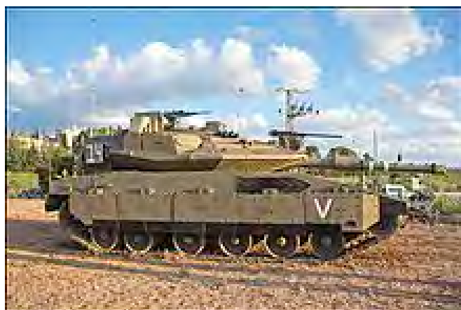
A profile of a Merkava Mk 4M tank, armed with an an IMI 120 mm gun , a M2 Browning .50-cal, a 7.62×51 mm NATO commander's FN MAG , and equipped with the Trophy active protection system .
