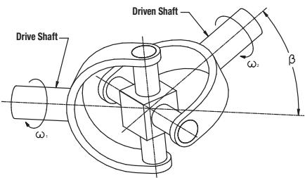
The average angular displacement and velocity is uniform. That is, if the driving yoke rotates one revolution, the driven yoke also rotates one revolution. However, during this one revolution, the incremental angular displacement and instantaneous angular velocity and acceleration are not transmitted uniformly through the joint. The angular displacement of the driven yoke during one revolution lags and leads the driving yoke twice.
