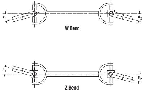
Synchronous rotation of the drive and driven shafts is possible provided that all three of the following conditions are met:
