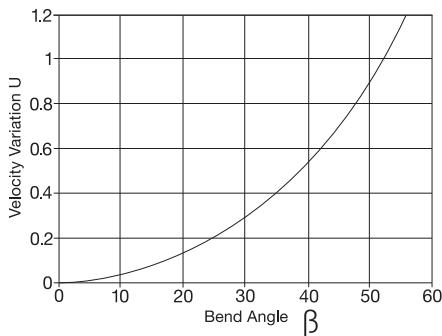
As a result of the non-uniform motion of a universal joint, few applications are suitable for a single universal joint. However, by placing two universal joints in tandem the irregularities of a single joint can be compensated. By arranging the two universal joints in either a "Z" or "W" bend configuration with joint angles  $\beta_1$  and  $\beta_2$ , equal, the velocity variations developed in the first joint are in effect cancelled by the velocity variations in the second joint.
