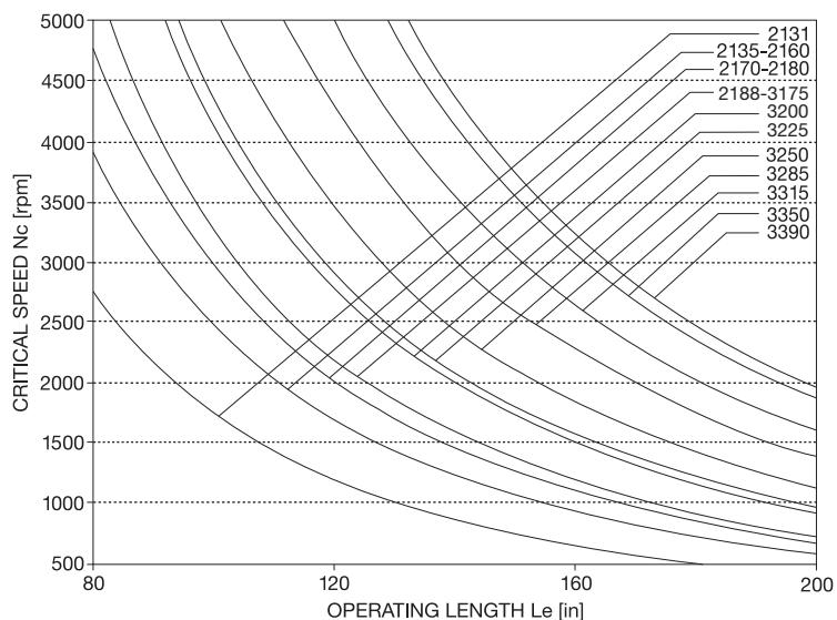
The speed limits on this page are only a guide. The actual limits are determined by the characteristics of the system in which the universal joint is installed.
