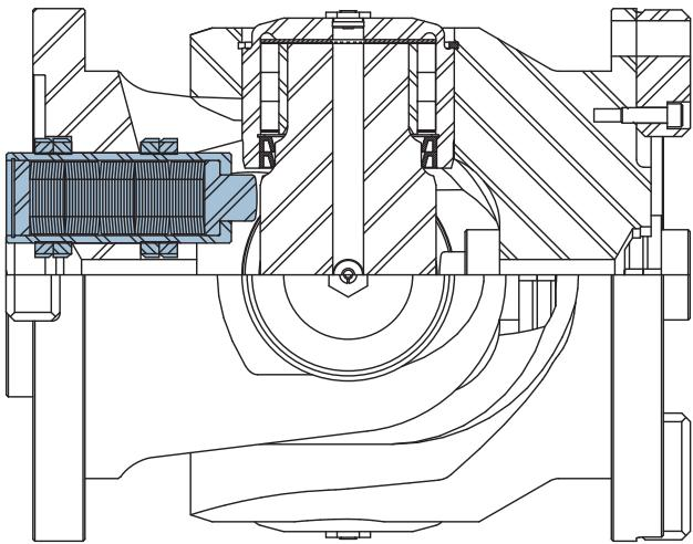
**Roll End Support Mechanism**
