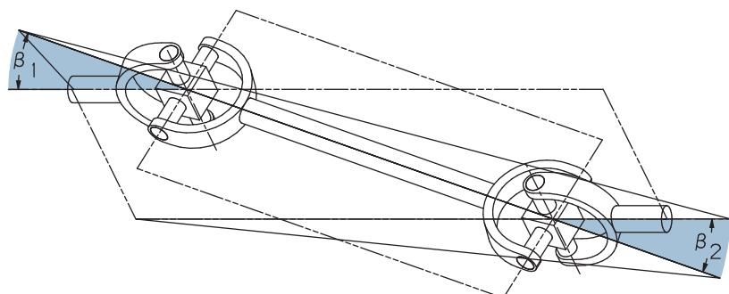
This ideal or phased arrangement will result in homokinetic operation of the universal joint driveline assembly. Failure to meet one or more of these requirements will result in some level of velocity fluctuation in the driven shaft. The acceptability of this velocity fluctuation is a function of the speed, system mass and the sensitivity of the application.
