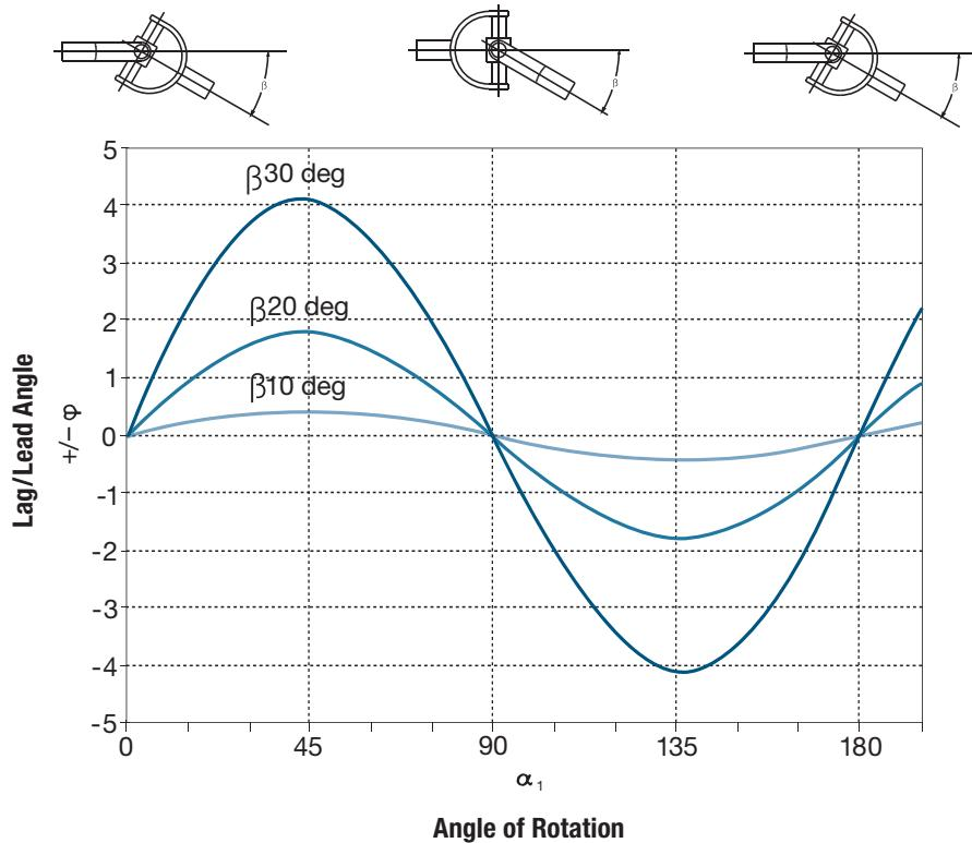
Lag and lead angle ( $\varphi$ ) as a function of angular rotation ( $\alpha$ ) of the joint and bend angle ( $\beta$ ).
