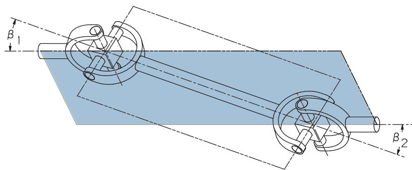
2. The bearing bores of the inboard yokes of the center section lie in the same plane.
