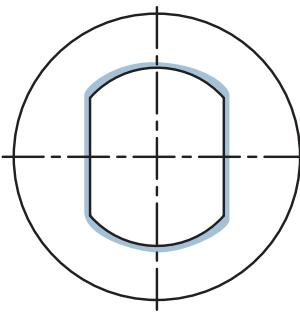
**Developed and Hardened Roll End Bore**
