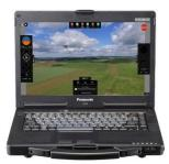
Orion system is controlled through a rugged Toughbook loaded with Elistair T-Planner software. Connected to Safe-T (Orion ground tether management system) through an ethernet cable, T-Planner is an easy-to-use and intuitive interface enabling the operator to control Orion, the XDM camera and Safe-T.
