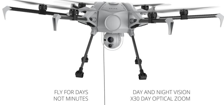
Powered from a ground source and through its patented micro-tether and built with industrial components, Orion is designed for long duration uses. Equipped with a gyro-stabilized multi-sensor full HD camera with day-light optical zoom X30 and an infrared camera, Orion is highly qualified for demanding and long staring missions in any day / night weather conditions.
