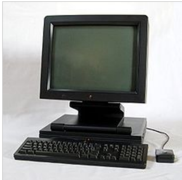
A NeXTstation with the original keyboard, mouse and the NeXT MegaPixel monitor
