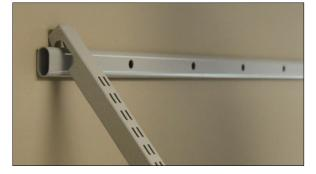
**STEP THREE:** Hang vertical slotted tube to the mounted oval support rail by inserting the top portion of the oval cutout to the top of the oval rail. Rotating the vertical rail to the wall to secure the rail to the horizontal oval support. To adjust, tilt the vertical rail away from the wall and slide to the desired position. No additional attachment is necessary to mount the vertical rail.
