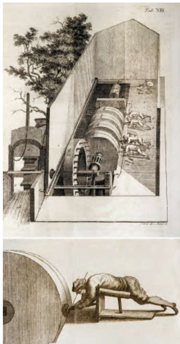
Figure 5. Top: This engraving from a 1776 book by Colosimo Collini, who explored the agate mining regions of southern Germany, shows a water mill cross-section in Oberstein along the Nahe River. The river current rotates the water wheel, which turns a geared axis. The gears turn the large sandstone wheels used to grind and form agate. Bottom: Another engraving illustrates in detail the arduous cutting process practiced by the German agate cutters, who used their bodies and the wheel to work the object. Courtesy of the Richard T. Liddicoat Library and Information Center.
