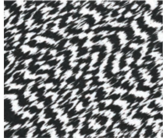
Figure 5. Extinction bands along chalcedony fibers, as seen with crossed polars in a petrographic microscope, reveal that the helical pitch is correlated among adjacent fibers. From Heaney et al. (1994).
