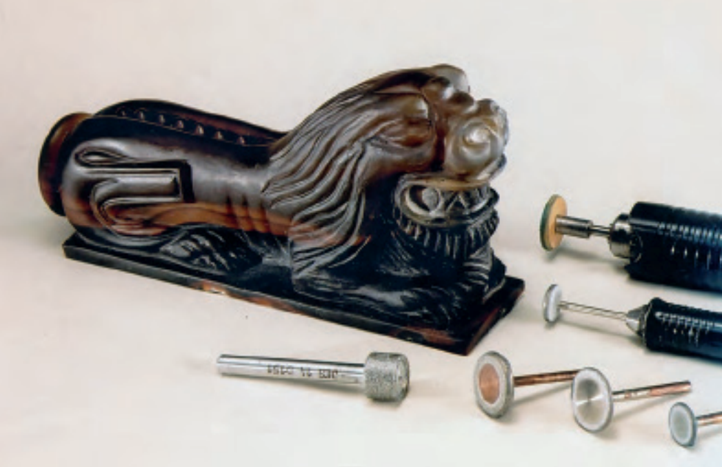
Figure 25. One of the lion armrest prototypes during the production process, pictured with some of the bits Van used in a Foredom flex shaft to carve the details.
