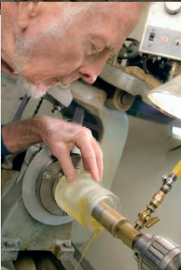
Figures 7a, b. Van's lathe, which he built inside his studio, was an adaption of commercial machining equipment, but with the motor slowed down for lapidary projects. Overset image: Van turns a rock crystal jar on the lathe. He uses a feeler gauge and stops to monitor depth as he grinds out the core.
