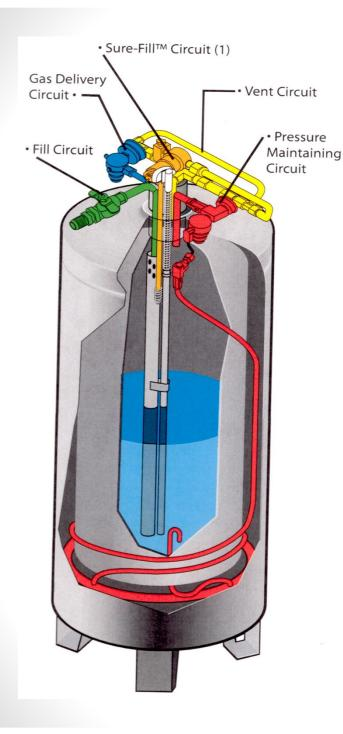
A bulk CO2 system is a single storage vessel that provides a continuous supply of CO2 to the beverage machine.
