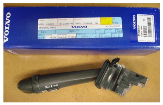
New switch shown. Note the electrical connector on the right and the gasket around the opening. Begin by removing the 3 torx screws from the bottom of the steering column cover.
