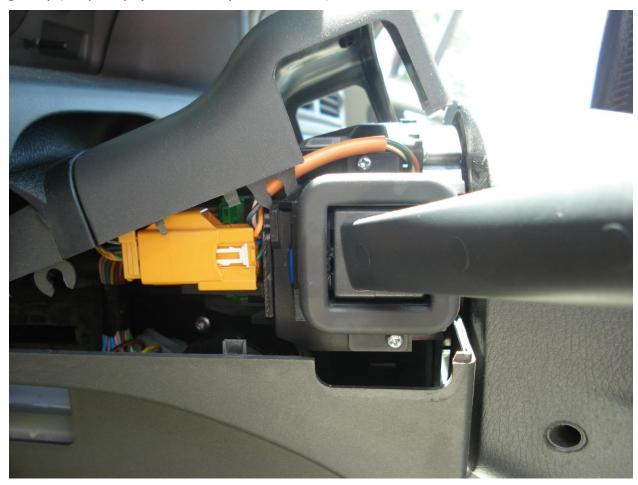
The switch is held in place by the 2 phillips head screws seen above. Undo the screws. The switch itself plugs into the 9 - pin electric socket, so it will take some moderate pressure (and a bit of working up and down) to get it free.
