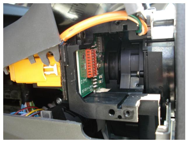
Installation is the reverse of removal. It will take some pressure to get the electric connector to seat. The screws are there to hold the switch in place. Get it seated first, then install screws.
