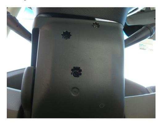
With those screws removed, pull down the bottom cover.
