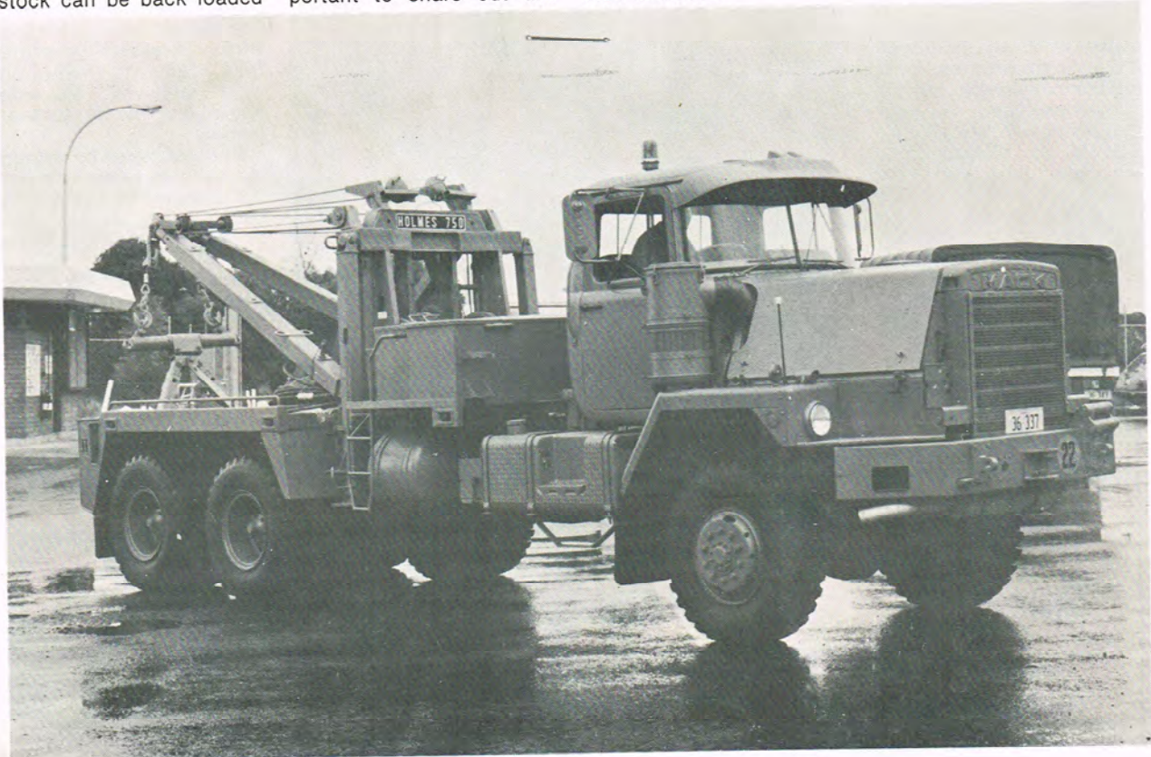
The Mack RM6866RS 6 x 6 is the basis of the Australian Army's new recovery vehicle. A Holmes 750 wrecker unit is mounted to the Mack to give a vehicle with the capacity to recover the complete range of military Class B vehicles. Mack Trucks Australia is supplying the Australian Army with 30 of these recovery vehicles.
