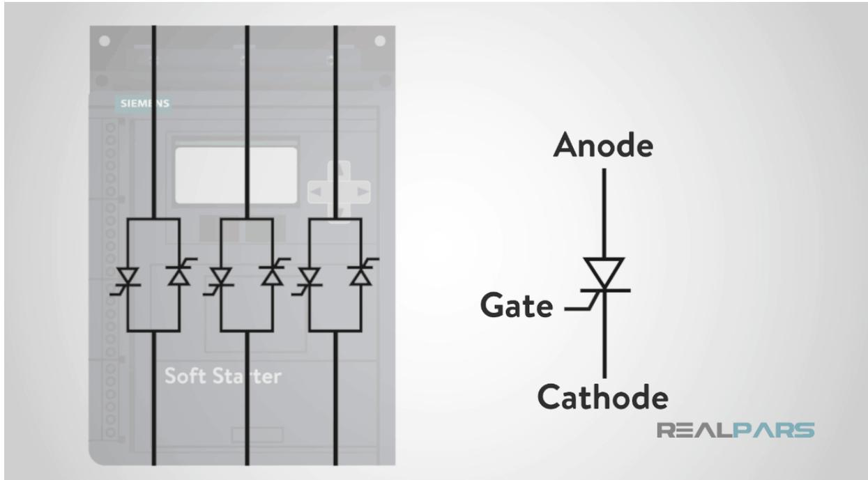
These internal pulses limit the applied voltage to the motor slowing down inrush current. The pulses are sent based on ramp time so the current will be slowly applied to the motor. The motor, attached to the soft starter, will start up at a nice smooth current and top out at the preset maximum speed.
