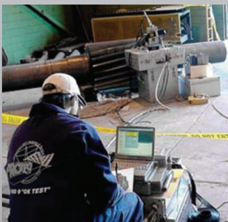
Fig. 7: Measuring residual stress on a component in the field
