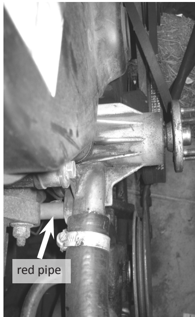
11. The left bolt of previous photo holds the red pipe going into arm of waterpump.
