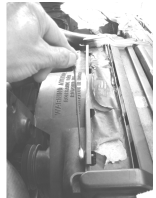
4. Remove 2 8-mm machine screws from top of radiator bell housing
