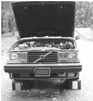
1. Drive car onto ramps. Set handbrake. Chock rear wheels.
