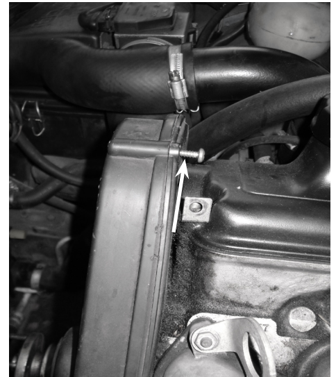
12. Remove top 1/2 of timing belt cover to get to last bolt in waterpump. First remove Phillips screw (arrow) back of top cover.
