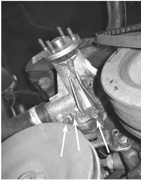
10. Loosen 3 bolts on bottom (arrows). Left bolt has nut on back. Middle and right bolts thread into engine block. Compare with step 22.
