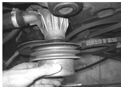
8. Pull waterpump pulley off. You may have to slip the fan belt off the power assist pump to make it easier; leave other end of belt on crankshaft pulley.
