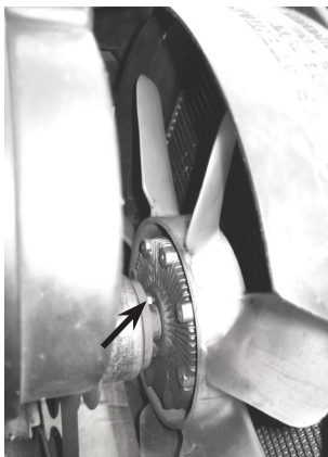
5. Dismantle fan/clutch assembly by removing 4 10-mm nuts (arrow) using open end wrench.
