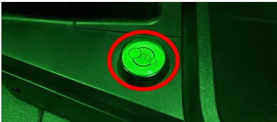
3. If the issue persists, remove the trackers from the player's footwear, turn them OFF then ON by holding the power button for 5 seconds, and clip the trackers back into the footwear
