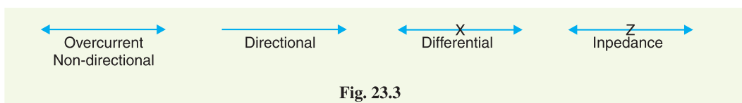
Fig. 23.3 shows the symbols indicating the various types of relays.
