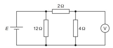
The voltmeter has a very high resistance and reads a potential difference  $V_{\rm out}$ .
