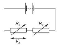
The variable resistors have resistances  $R_X$  and  $R_Y$ .  $V_X$  is the potential difference across resistance  $R_X$ .
