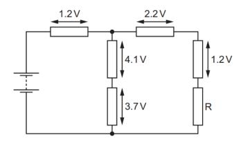
The potential differences across five of the resistors are labelled on the diagram.
