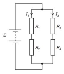
The currents  $I_1$  and  $I_2$  in the resistors are as shown.
