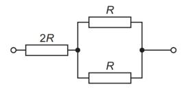
What is the ratio  $\frac{\text{total resistance of network 1}}{\text{total resistance of network 2}}$ ?
