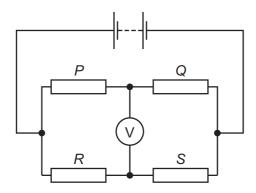
The voltmeter reading is zero.
