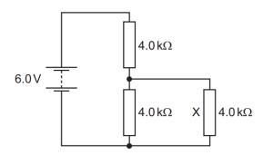
Each resistor has a resistance of  $4.0 \, k\Omega$ .
