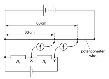
One terminal of a galvanometer is connected to point X. The galvanometer reads zero when its other terminal is connected to a point that is a distance of 60 cm from one end of the potentiometer wire.
