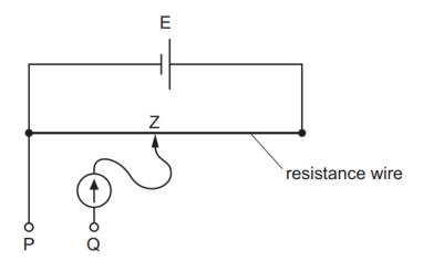
Z is a connection that may be made at any position along the resistance wire. A galvanometer is connected between Z and a point Q.
