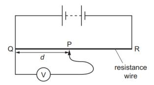
The potential difference (p.d.) *V* between the sliding contact P and end Q of the wire is measured using a voltmeter. The sliding contact P is moved from end Q to end R of the wire. Sliding contact P is distance *d* from Q.
