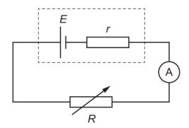
When R is  $10\Omega$  the ammeter reads 0.3 A.
