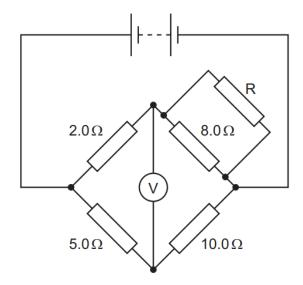
The voltmeter reading is zero.
