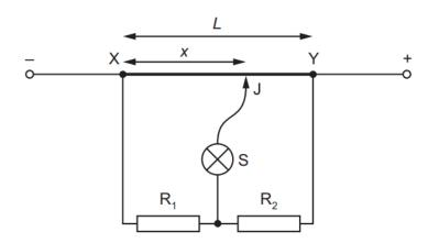
J is moved along XY to a point at which the lamp is off. This point is at a distance x from X.
