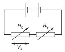
The variable resistors have resistances  $R_X$  and  $R_Y$ .
