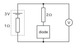
A high-resistance voltmeter is connected across the diode and resistor.
