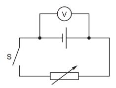
When switch S is open, the voltmeter reads 1.5 V. The switch is then closed and the variable resistor is adjusted to have a resistance of  $4.0\,\Omega$ . The voltmeter now reads  $0.75\,V$ .
