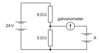
The galvanometer has a current reading of zero.
