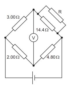
The reading on the voltmeter is zero.
