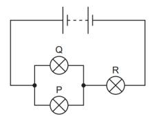
The filament wire in lamp Q breaks so that it no longer conducts.
