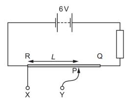
Terminal X is connected to fixed point R. Terminal Y is connected to point P, a connection that may be made at any position along the wire. *L* is the distance between R and P.
