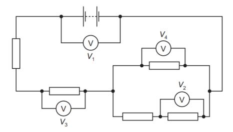
The reading  $V_1$  is 8.0 V and the reading  $V_2$  is 1.0 V.
