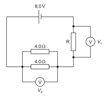
The reading  $V_1$  is 4.0 V and the reading  $V_2$  is also 4.0 V.
