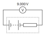
When a resistor of resistance  $11.0\,\Omega$  is connected in parallel with the battery, the voltmeter reading changes to  $8.800\,V$ .
