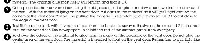
Fold over the edges of the material to glue them in place on the backside of the vent door. Do not glue the center area of the vent door. The material is intended to float on the vent door. Remember to pull tight like stretching a canvas. Start at one side and attach the darts to the back and move to the opposite side as well as the third and forth side.
