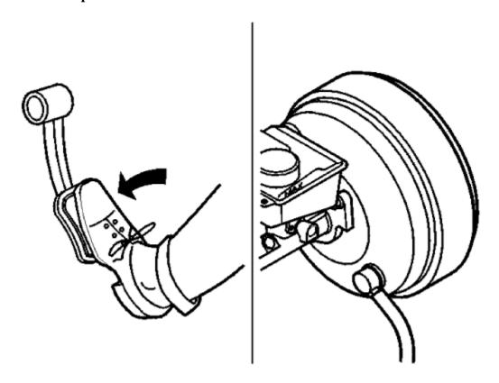
Check if there is a vacuum to the power brake booster. Do this by removing the hose from the check valve.
