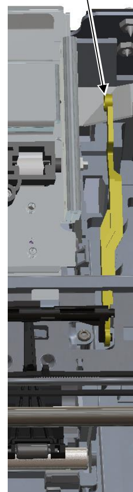
Pinch Roller Release
