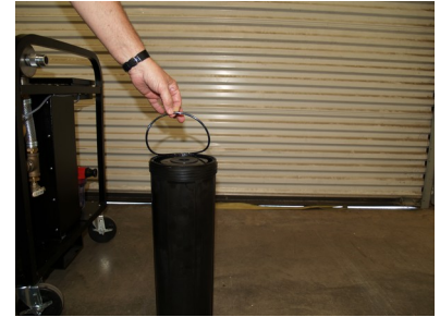
Inspect o-ring Replace canisters
