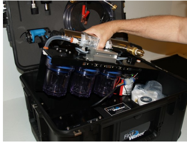
Lift out filter housing
