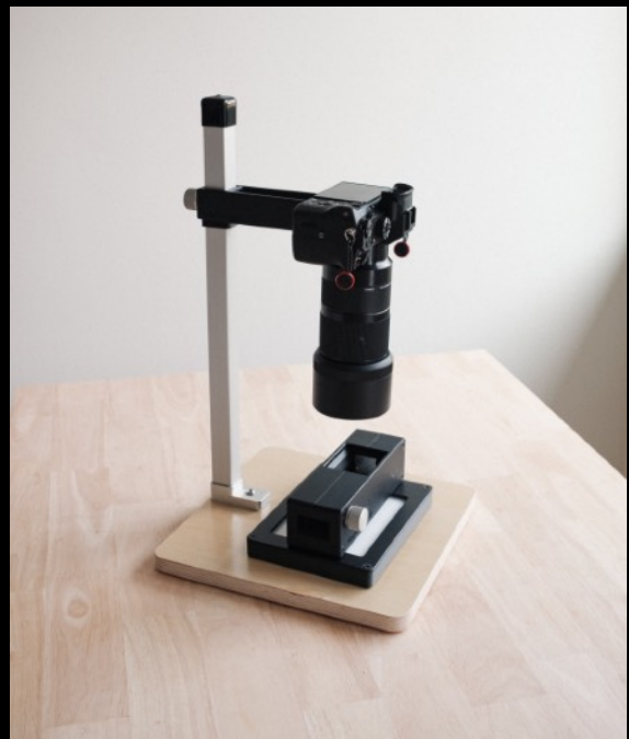
A basic Camera Scanning Setup comprised of the Basic Riser, The Film Carrier MK1, and a Basic Light.
