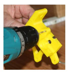
Re-drill (3 mm) the side hole of the extruder.
