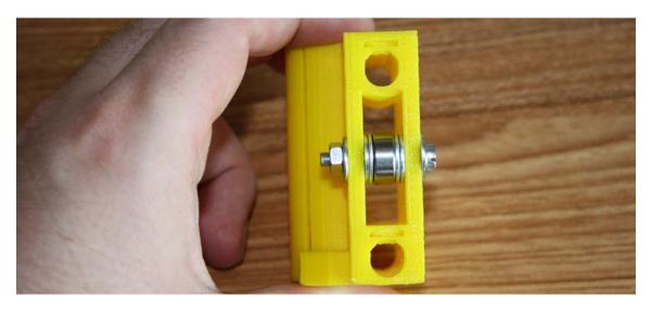
Slide an M4x25 bolt with an M4 washer through the X End Idler, put two washers, a small ball bearing and two more M4 washers in the middle. Fix the bolt with an M4 washer and an M4 nut.
