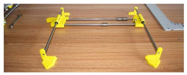
Slide one 320 mm smooth rod through the bearings of the X End Idler, and another 320 mm smooth rod through the bearings of the X End Motor. Fix the ends with the Z Axis Top and Bottom parts. Take two 370 mm smooth rods. Put two LM8UU bearings on the upper rod and one on the other rod. Connect the smooth rods to the X End Idler and Motor parts.
