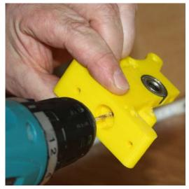
Re-drill (3,5 mm) the bottom hole of the extruder.
