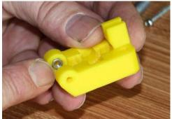
Heat up an M3 nut and place it into the side of the Gidler.
