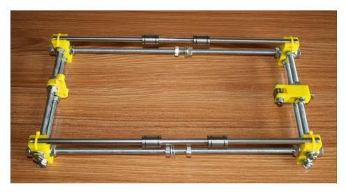
Slide all the ends through the Y corners of the vertical sides. Fix them with a washer & nut (hand-tight). Fasten the smooth rods with four tie-wraps.
