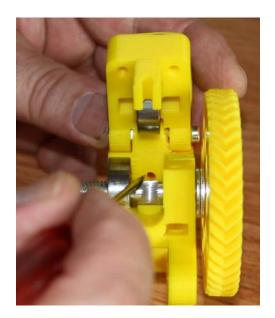
Slide a hobbed bolt through the big gear. Put 2 M8 washers on the hobbed bolt. Now slide it through the side of the extruder. Make sure the hole, pointed in the picture, is in line with the teeth's of the hobbed bolt. Put a large ball bearing next to it.
