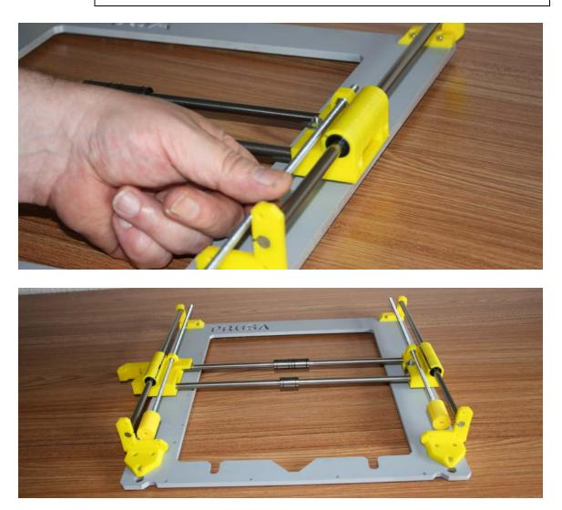
Place an M5 nut in the X End Idler & Motor. Turn the threaded rods until in position.
