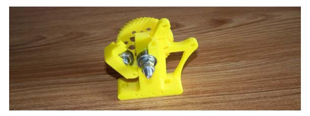
Fix the hobbed bolt with an M8 washer and 2 nuts (next to the large ball bearing of step 6-5).
