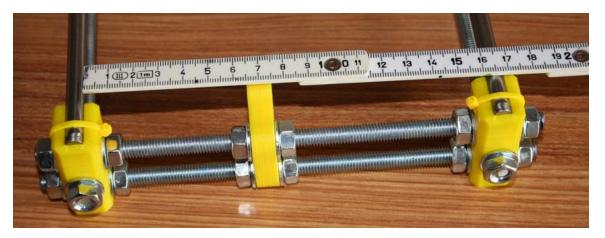
Measure the distance between the smooth rods. It should be at approximately 16,2 cm. Make sure the Y-carriage runs smoothly up and down. Tighten the outer nuts with a wrench and the Y Bushings of the Y-carriage with a screwdriver.
