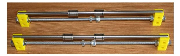
Take two 380 mm threaded rods. Place an M8 nut, two M8 washers, and another M8 nut in the middle of each threaded rod. Fix the threaded rods to the Y corners with another nut and washer (hand-tight) on either side. Slide two LM8UU bearings onto the two 360 mm smooth rods. Push the smooth rods carefully on top of the Y corners.
