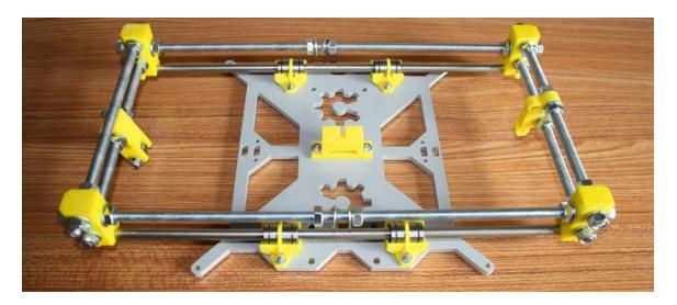
Connect the Y-carriage to the Y-axis frame. Carefully place the LM8UU bearings in the Y bushings and fix them with four tie-wraps.
