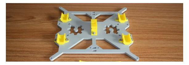
Mount (hand-tight) the four Y Bushings, with eight M3x16 bolts, 16 M3 washers and 8 M3 nuts, to the Heated bed Mount. Place the Y Belt Holder on the middle of the Heated bed Mount and fix it with two bolts, four washers and two nuts.
