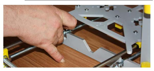
Mount the Y-Axis frame to the Aluminium frame by tightening the M8 nuts.
