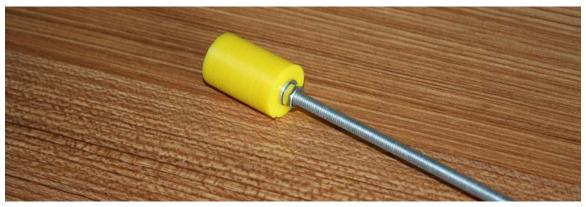
Turn the two 300 mm threaded rods in the other opening of the Z Couplers. Fix them with an M5 washer and nut
