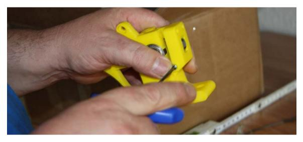
Connect the gidler to the extruder with an M3x25 bolt.
